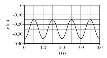
An unstretched ideal spring hangs vertically from a fixed support. A 0.4 kg object is then attached to the lower end of the spring. The object is pulled down to a distance of 0.35 m below the unstretched position and released from rest at time t = 0. A graph of the subsequent vertical position y of the lower end of the spring as a function of t is given above, where y = 0 when the spring was initially unstretched.
